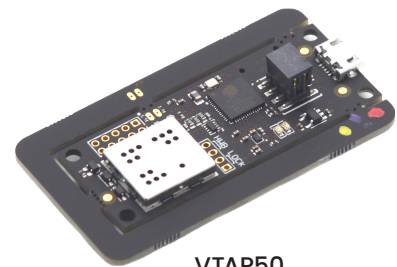
VTAP50 20mm x 52mm using external antenna 32mm x 58mm with own antenna
